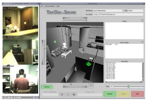
Figure 9. ResiSim indicates activated motion sensors with green orbs.
