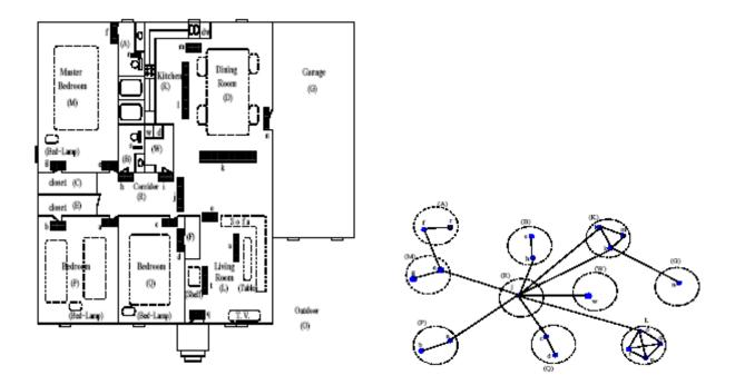
Figure 5. (a) Typical floor plan of MavHome architecture, (b) Graph representing connectivity of sensor zones
